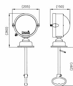
All dimensions in Millimetres **Base Fittings** MK1 – 3 holes Ø8 on a 80.0 P.C.D. M12 – 3 holes  $\emptyset$ 6.4 on a 108 P.C.D. with a centre control clearance hole Ø45.
